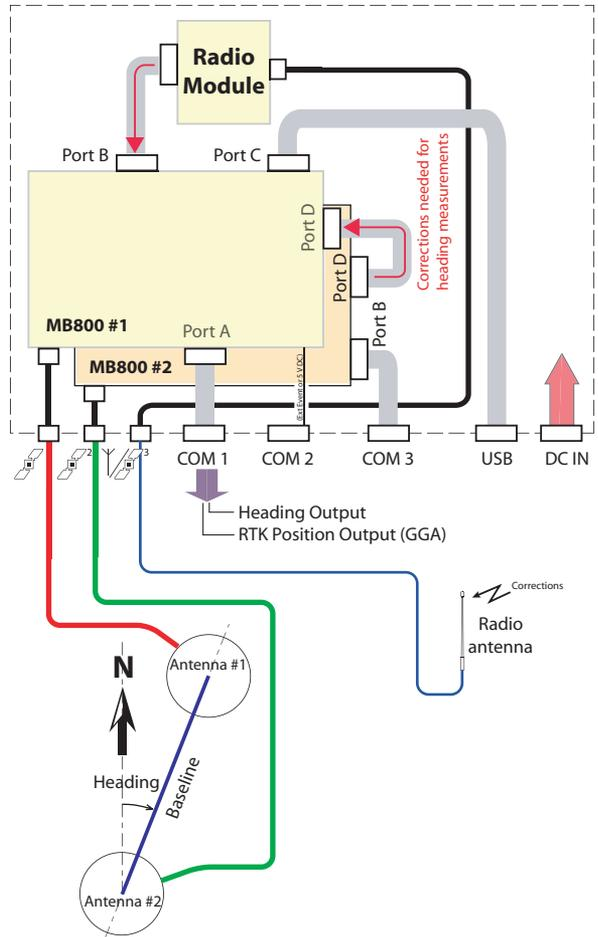
**Heading Output.** Make sure you are sending your commands directly to board #2 through **COM 3** (default baud rate: 115200).
