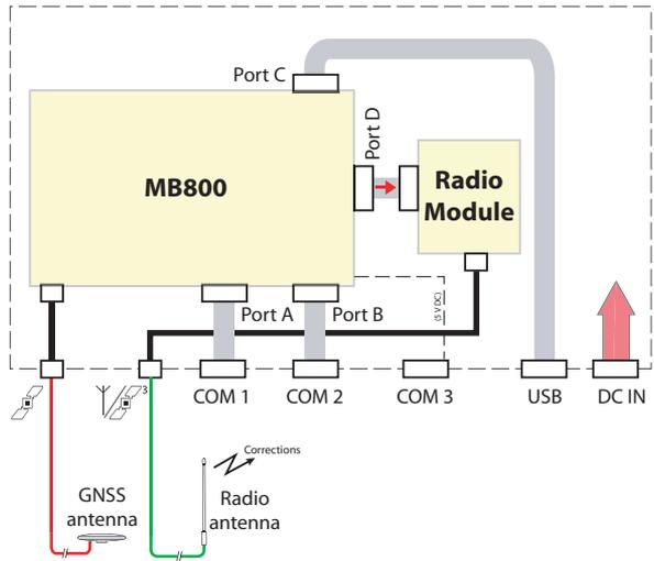
Follow the same configuration instructions as those provided for *RTK Base on page 35*, except that the generated corrections messages should be routed to the internal radio via MB800 port D. For example, run this script to set an RTCM3.0 base:
