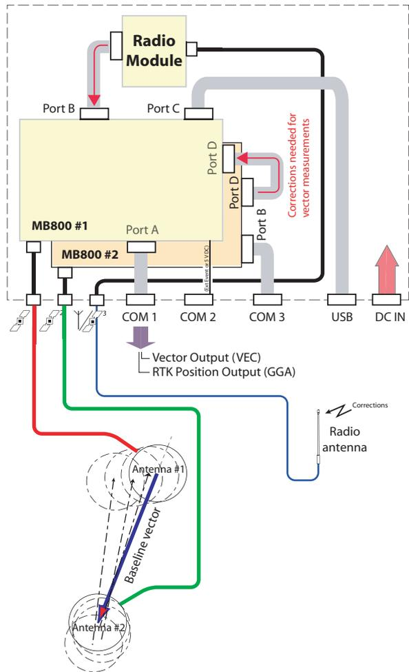
**Vector Output.** Make sure you are sending your commands directly to board #2 through **COM 3** (default baud rate: 115200).
