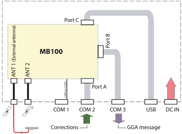
1. Run the following command to choose COM 2 (internal port A) as the port acquiring incoming differential corrections (this is the case by default).
