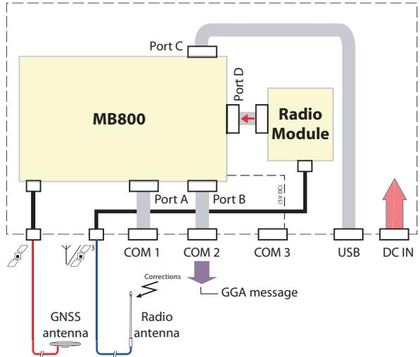
1. Run the following command to choose internal port D as the port acquiring incoming differential corrections.
