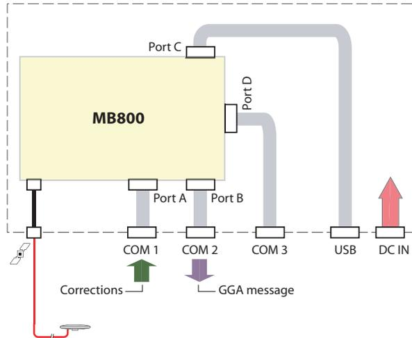
1. Run the following command to choose COM 1 (internal port A) as the port acquiring incoming differential corrections (this is the case by default).
