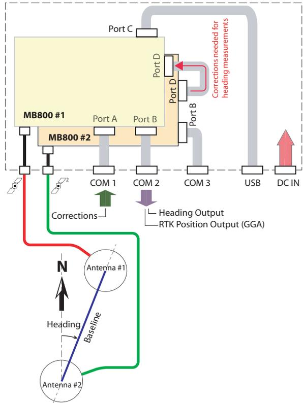
**Heading Output.** Make sure you are sending your commands directly to board #2 through **COM 3** (default baud rate: 115200).
