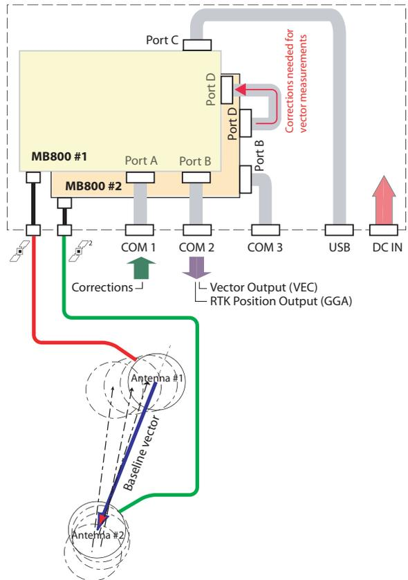
**Vector Output.** Make sure you are sending your commands directly to board #2 through **COM 3** (default baud rate: 115200).
