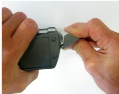
If for some reason you need to remove a bar, squeeze it as shown on the picture below. By squeezing the bar, you temporarily deform the aluminum plate thus releasing it from the case:
